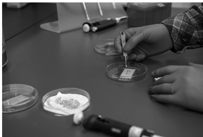
Figure 6: Making the perfect sample is at the intersection of materials science and biological research. EM sample preparation on metal grids or other materials requires conductive, flat surfaces with reliable physical properties under a variety of temperature extremes.
