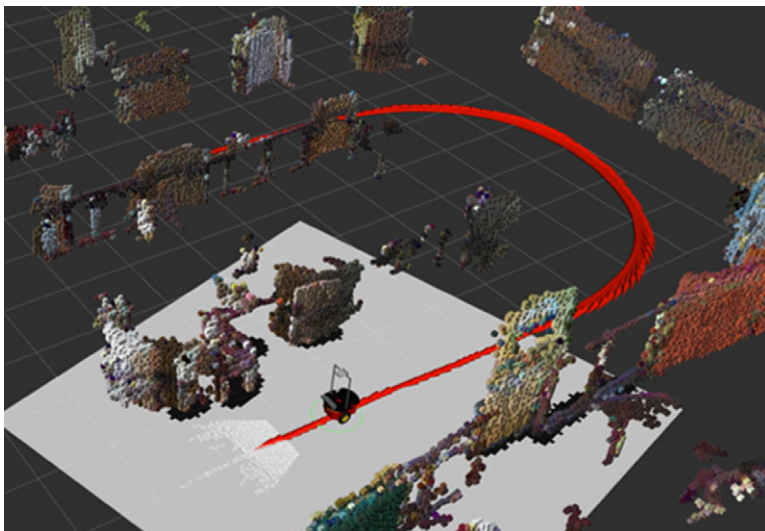
Figure 3. Map generated by RTAB-Map using visual-SLAM, and the path (red-colored curve) planned by the robot.
