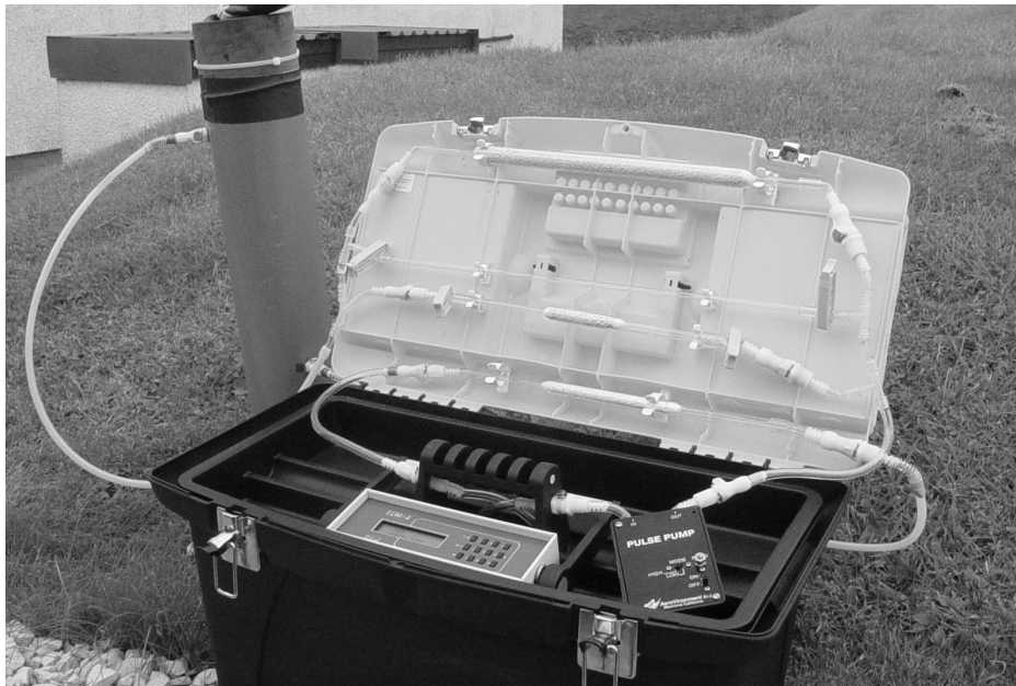
Figure 2 The molecular sieve sampling system in field operation. The chamber is for demonstration purposes only.
