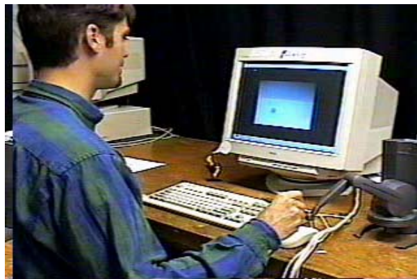
Fig. 3. J. Cummings using force feedback pen to guide magnetic bead through liquid sample.
