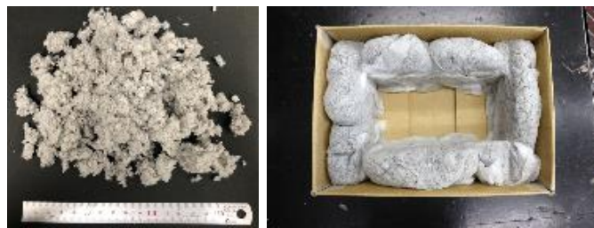
Figure 6. Sound-absorbing material placed inside the box
