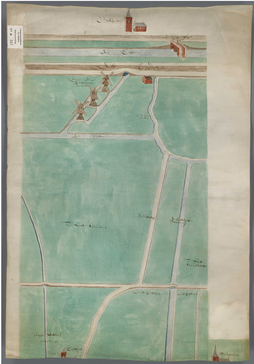
FIGURE 10.5b Set of three windmills near Reeuwijk. Author and date unknown. Three windmills are required to pump the water from the polder into the drainage canal surrounding it. (Source: Archive of the Hoogheemraadschap Rijnland number A-0517. (NL-LdnHHR, Collectie kaarten, A-0517) (Reproduced under CC-BY-SA)
