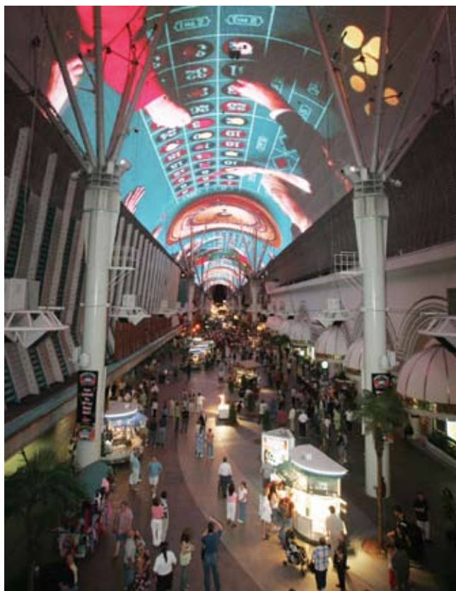
Figure 7. One of the largest LED displays in the world, on Fremont Street in Las Vegas, Nevada. The picture changes continuously. The initial display contained 2.1 million filament light bulbs, which constantly needed to be replaced because of failure. The new display, opened in 2004, contains 12.5 million LEDs.
