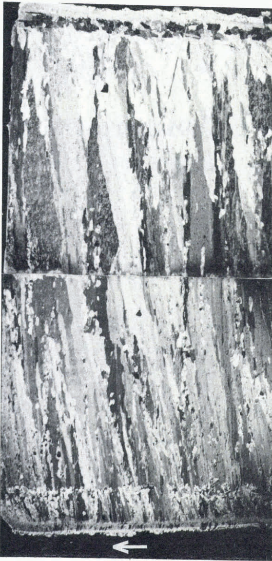
Fig.8. Vertical thin section in the x-plane from run 8. Columnar growth extends from the ice surface to the base of the ice. There is a deflection of the grains upstream into the current, the direction of which is shown by the arrow.
