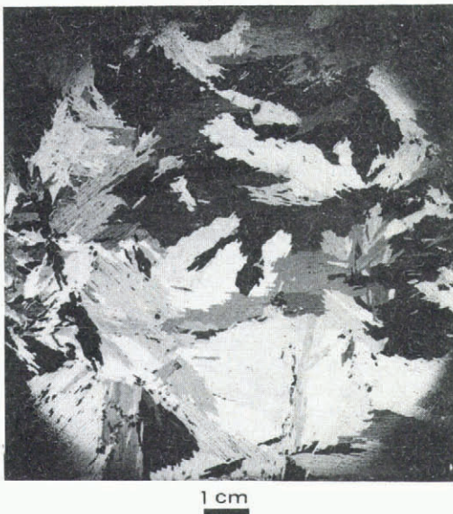
Fig.6(a). Horizontal thin section from run 7 (saline-no forced flow) taken 15 cm below the ice surface. Note the well-defined platelets.
