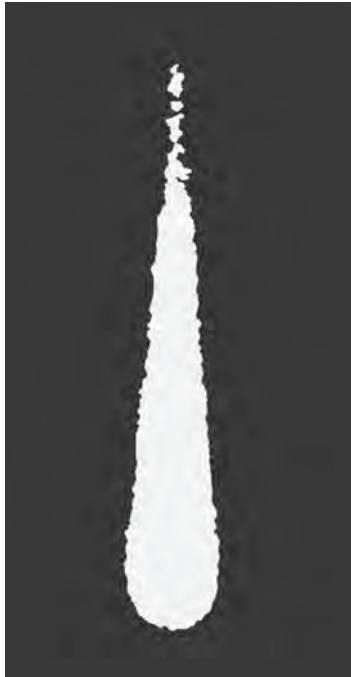
Fig. 5.9. Photographic reproduction of an electron avalanche [13, 16, 31, 32]. The photo shows the form of the avalanche. It was made visible in a cloud chamber (see Chap. 6) by droplets which had condensed on the positive ions.
