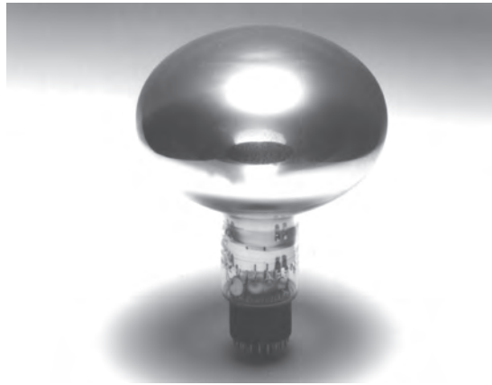
Fig. 5.33. Photograph of an 8-inch photomultiplier (type R 4558) [117].
