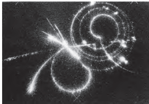
Fig. 6.7. Interaction of an antiproton with a neon nucleus in a streamer chamber producing – among others – a positive pion which decays into a muon yielding eventually a positron which escapes from the chamber [18].
