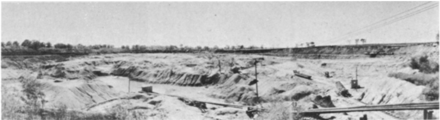
PLATE 1.—Panorama across a semi-plastic and semi-flint clay pit near Mexico, Missouri. The sump hole and low spots were filled with fire clay and represent depressions in the pre-Cheltenham topography; the “rises” are old hills rising above the basins. The sump hole contained fire clay to a depth of approximately 60 feet. A thin layer of conglomeratic sandstone lay between the fire clay and the underlying limestone. Photograph furnished by courtesy of the A. P. Green Fire Brick Company.
