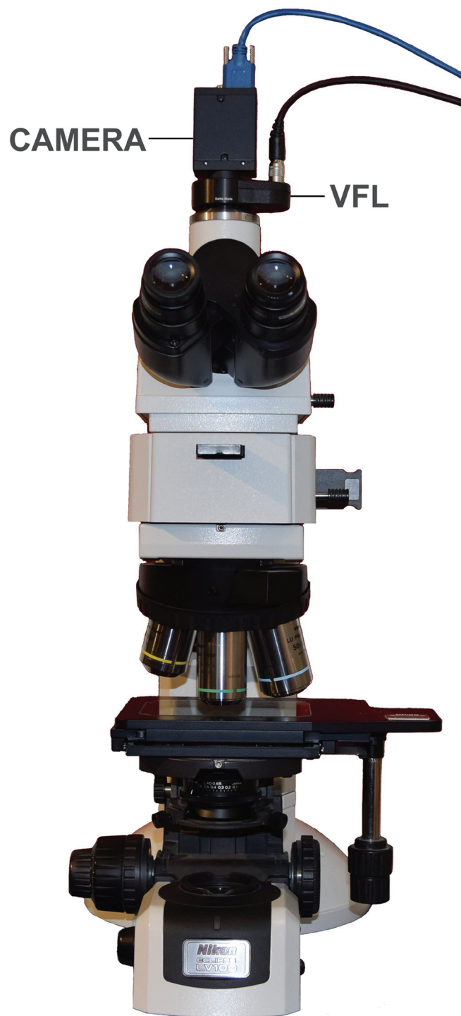
Figure 1: One embodiment, i.e., version, of the patented invention showing a camera and a variable focus lens (VFL) mounted on the trinocular port of a Nikon Eclipse LV100 microscope. The camera is connected to a personal computer, and the VFL is connected to computer-controlled custom driver electronics that are described in the patent of Figure 2.
