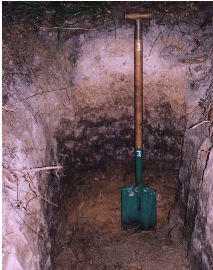
Figure 3 Humus horizon of fossil soil formed on loess deposits (top of the Wodzisław Hummock, near Wola Chroberska).
