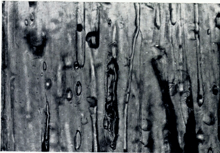
Fig. 8. Young sea ice. Interior faces in Tyndall figures are visible. Drainage-channel development from a brine pocket and Tyndall-figure migration
