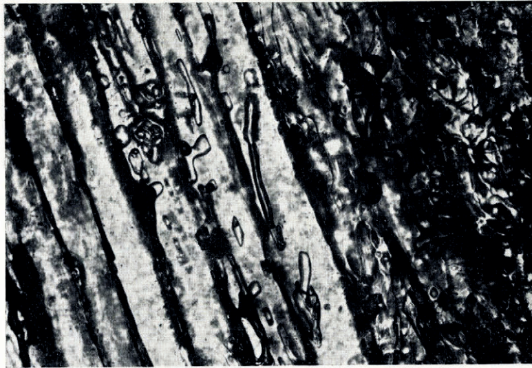
Fig. 6. Young sea-ice section. Tyndall-figure migration within platelets and the brine pocket between platelets is apparent. Platelets are \sim 0.5 mm. thick
