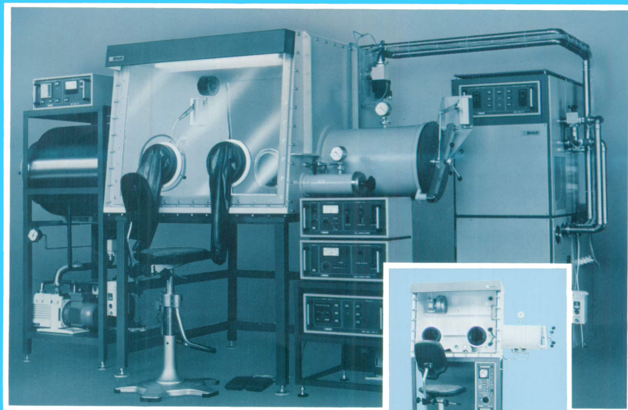
Above: Model MOD 200 Glove Box with two work stations, purifier MB 200 G, allowing for 24-hour operation. Vacuum oven, mini-chamber, moisture analyzer, oxygen analyzer, box and ante-chamber control with solid state safety device. Right: Model MB 120 or 150 single station Glove Box with integrated gas purification system.
