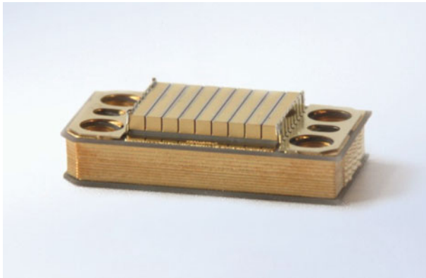
Figure 10. Photograph of JenLas® QCW Cool laser diode stack with 8 laser bars spaced at 1.7 mm pitch.
