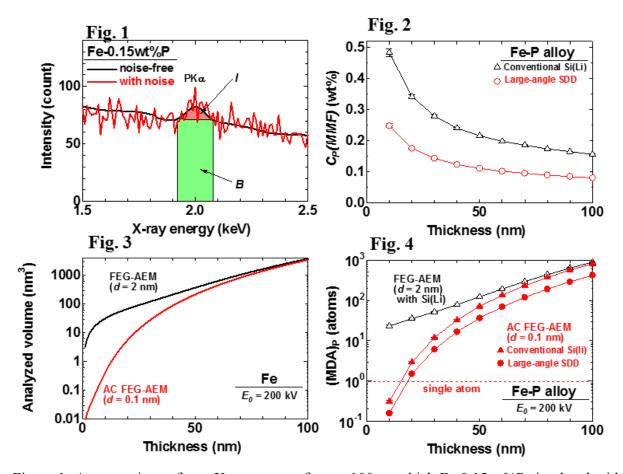
Figure 1: A comparison of two X-ray spectra from a 100-nm-thick Fe-0.15wt%P simulated with and without noise in a 200 kV instrument for 100 s.
