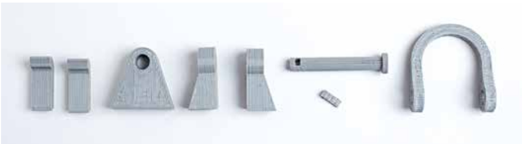
Fig. 6. and Fig. 7. Model of the lewis assembled (left) and disassembled (below), made by the authors
