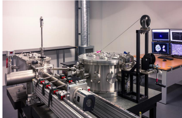
Figure 1. The SiriusXT compact Soft X-ray microscope, with an overall footprint of 3m x 2m.
