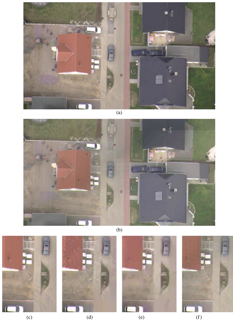
Fig. 11. Subjective image quality comparison for different video codecs and different very low bit rates (350 m sequence, 150–500 kbit/s). (f) ROI HEVC is proposed. Best viewed in pdf. (a) Original frame (whole frame). (b) ROI HEVC en- and decoded (whole frame, 300 kbit/s). (c) Original. (d) AVC 500 kbit/s. (e) HEVC 150 kbit/s. (f) ROI HEVC 150 kbit/s.
