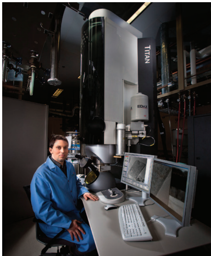
Figure 2: EMSL’s aberration-corrected FEI Titan scanning/transmission electron microscope (S/TEM) provides high-resolution imaging with sub-angstrom resolution and spectroscopic capabilities.
