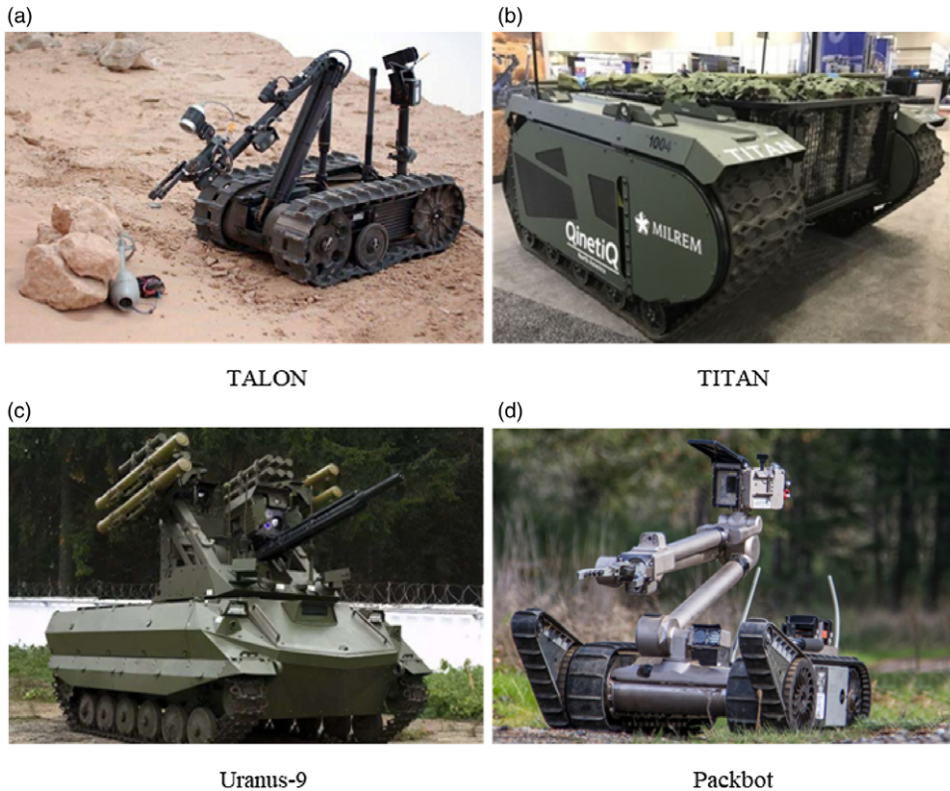
Figure 6. Tracked type UGV platform: (a) the Foster-Miller's TALON [19]; (b) the Qinetiq Titan [20]; (c) Russia UGV of Uranus-9 [21]; (d) American iRobot of Packbot [22].
