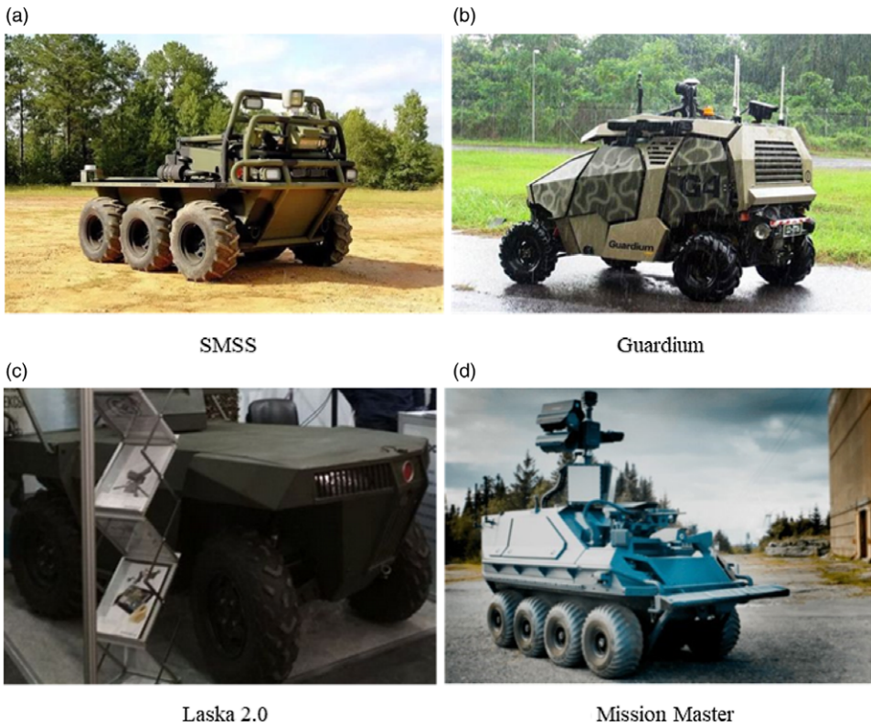
Figure 5. Wheeled type UGV platform: (a) the squad mission support system (SMSS) [5]; (b) Israeli off-road platform Guardium [6]; (c) the Laska 2.0 URP [7]; (d) Rheinmetall Mission Master [8].
