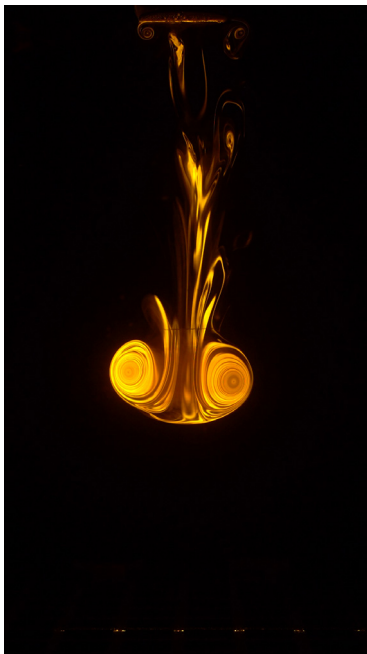
Figure 1. Visualisation of a ring vortex moving steadily into (a,b) a quiescent flow and (c,d) a turbulent field generated by an oscillating grid, both at 4.6 and 17.0 s, respectively, after vortex generation. The Reynolds number of the initial vortex, based on velocity and distance between the vortices, is 3200. Experimental parameters correspond to experiment T in table 1. The image is 50 cm wide.
