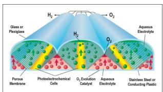
**Figure 4.** Conceptual design of photoelectrochemical water-splitting system with light concentration. The cylindrical pipes serve as light concentrators and gas collectors.  $H_2$  gas (green) is formed at the illuminated photoelectrode and  $O_2$  gas (red) at the counterelectrode. Ion transport between pipes is accomplished using porous membranes. Adapted with permission from Reference 30. ©2008, Macmillan Publishers.
