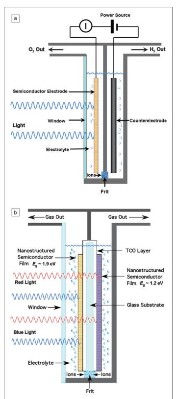
**Figure 1.** (a) Photoelectrochemical cells with single bandgap and (b) dual bandgap absorber (tandem). Blue and red light are absorbed by the large bandgap (front) and small bandgap semiconductors (back), respectively.  $E_{\rm g}$ , bandgap energy; TCO, transparent conductive oxide.
