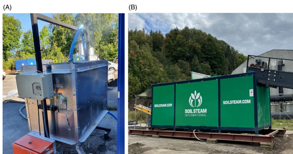
Figure 1. (A) The steaming prototype device (test box) used in the second experiment. (B) The prototype steaming machine (S30) used in the third experiment. Photos: (A) Ewa Orlikowska; (B) Soil Steam International AS.
