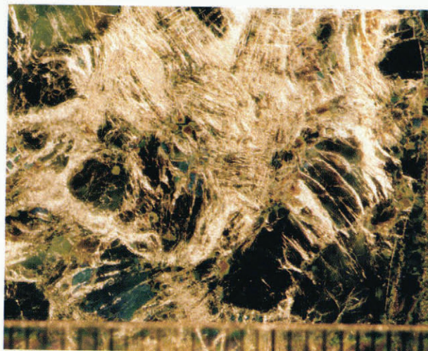
Plate 5. Enlarged view of thin sections from Plate 4. Samples were deformed to strains of 4% (a), 10% (b) and 44% (c). Scale is in mm.
