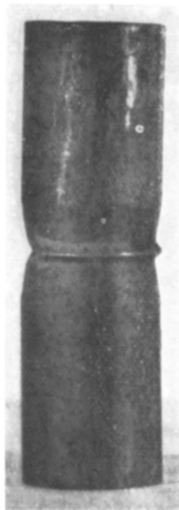
FIG 17 TUBE THAT FAILED IN COMPRESSION
