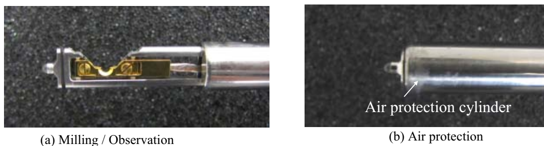
FIG.2 External view of cryo-air protection FIB-STEM compatible specimen holder of tip parts.
