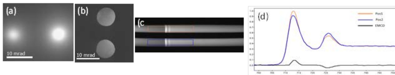
Figure 1: (a) Electron DP with the sample tilted in 2BC (b) the image of the DA (c) image of the two EELS spectra (d) EELS spectra extracted from (c) and their difference (EMCD) signal
