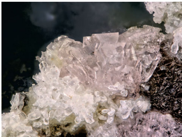
Figure 1. Pink naalasilite crystals with colourless crystals of anhydrite on holotype specimen 76282; the field of view is 0.68 mm across.
