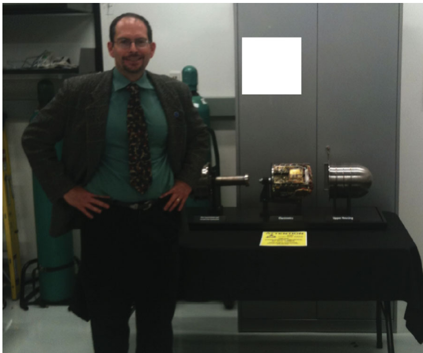
Figure 6. The author in front of a duplicate of the Galileo Probe mass spectrometer (on table) built by Hasso Niemann of the NASA Goddard Spaceflight Center. The detector is on the left; electronics in the center, and the upper housing on the right. Photo by M. Amato.
