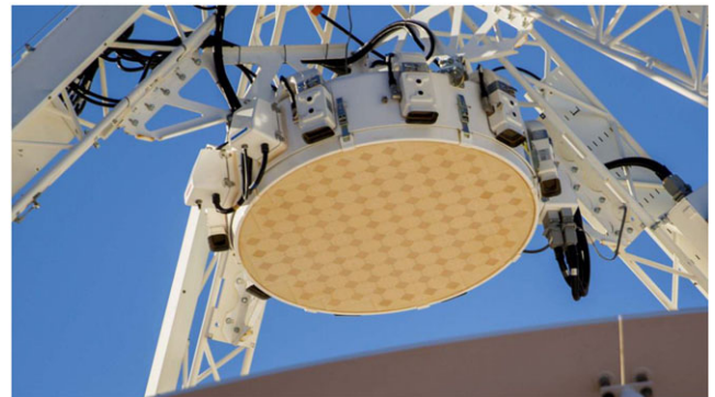
Figure 3. One of the phased array feeds. Each square on the chequerboard is an antenna element connected to two receivers. Photo credit: CSIRO
