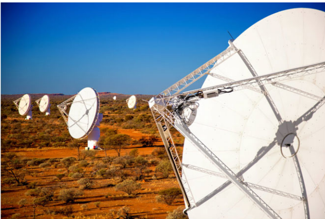
Figure 2. Some of the ASKAP antennas equipped with phased array feeds, located in the Murchison Region of Western Australia. Photo credit: CSIRO
