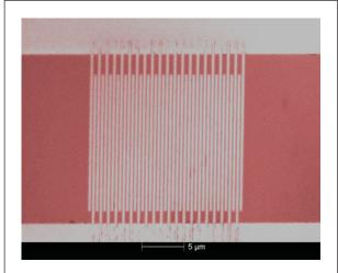
Colorized micrograph of an ultrafast single-photon detector made of superconducting nanowires. Electron beam lithography is used to pattern the nanowires (colorized vertical lines) on a thin film of tungsten-silicon alloy, which produces more reliable signals than the niobium nitride material used previously. *Credit*: Baek/NIST.
