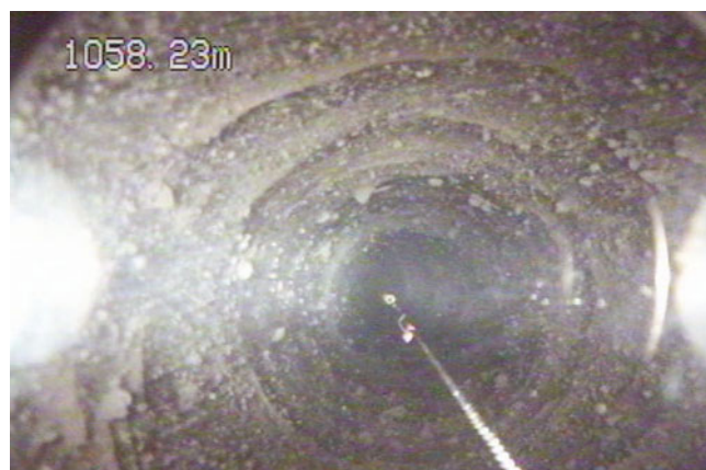
Fig. 14. Elevated debris content, with rocks sticking out from a rough borehole wall.
