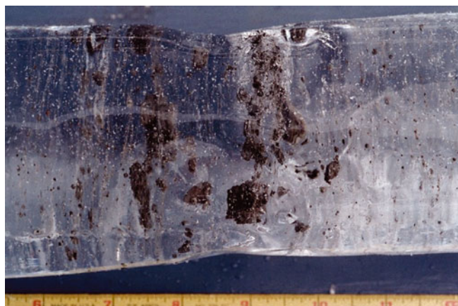
Fig. 4. Ice core with debris at same depth as in Figure 3. The ice-core diameter is 100 mm. The scale along the core is in inches.
