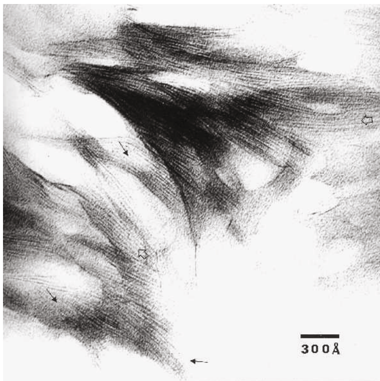
Figure 6. Ultrathin section of smectite treated with HDTMA ions equivalent to 0.8 times the CEC of the clay. The overall layer spacing is 17 Å, and is slightly curved, but spacings smaller or larger than 17 Å are observed. 14 Å (thin arrows) and 21 Å (open arrows) layer spacings are shown.
