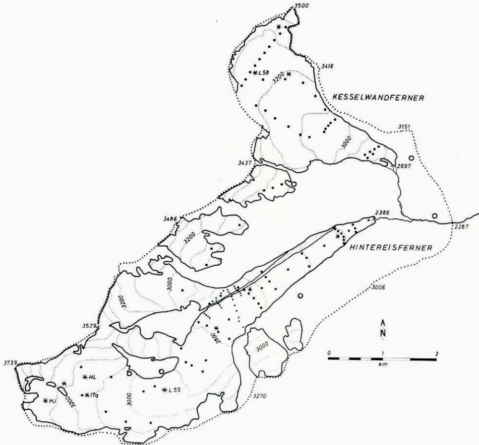
Fig. 1. The drainage area ( 26.6 \text{ km}^2 ) of the Hintereisferner and the Kesselwandferner, Ötztal Alps. Heights in metres a.s.l., interval of contour lines 100 m. Positions of ablation stakes (●), snow pits (★) and rain gauges (○) are shown for 1959
