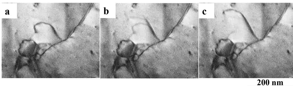
Figure 3. Bright field STEM image observation of dislocation slip in Cu thin foil at 600°C. ( a:0s, b:0.5s, c:1.0s)
