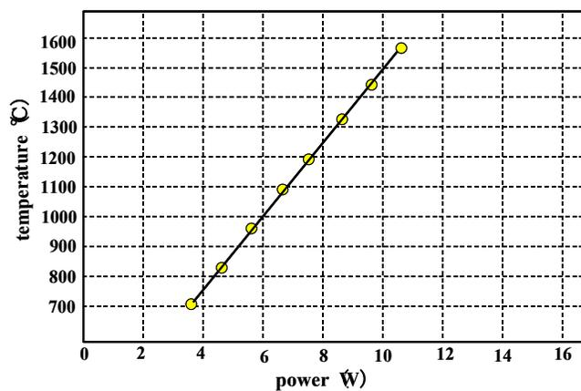
Figure 2. Heating temperature (°C) as a function of heating power (W)
