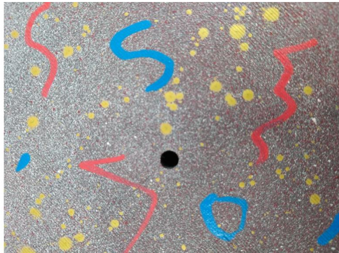
Figure 3: An example of the surface patternation applied to each test artefact prior to digitisation via photogrammetry.
