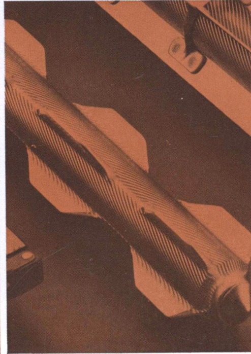
H.D.A. precision forgings in fuel elements for the U.K. Atomic Energy Authority.
