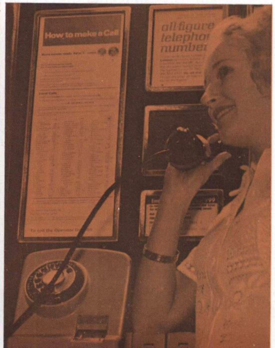
Casing of an S.T.D. coin box made at H.D.A.'s pressure die foundry.
