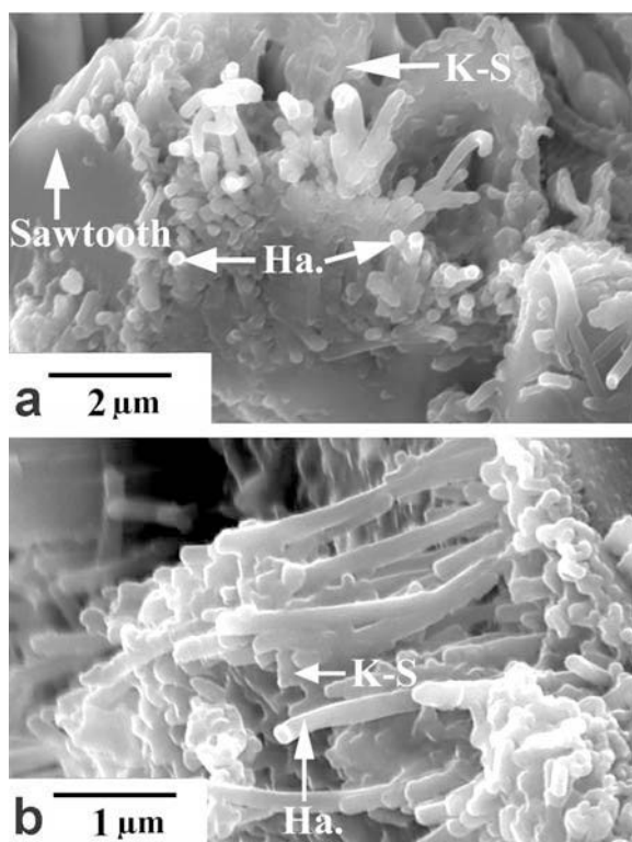
Figure 10. SEM observations of the last stage of the crystallization sequence on a (001) amphibole surface: (a) interstratified K-S (K-S) and halloysite (Ha.) on sawteeth, showing tubular halloysite; (b) tubular halloysite (Ha.) on interstratified platy K-S (K-S).
