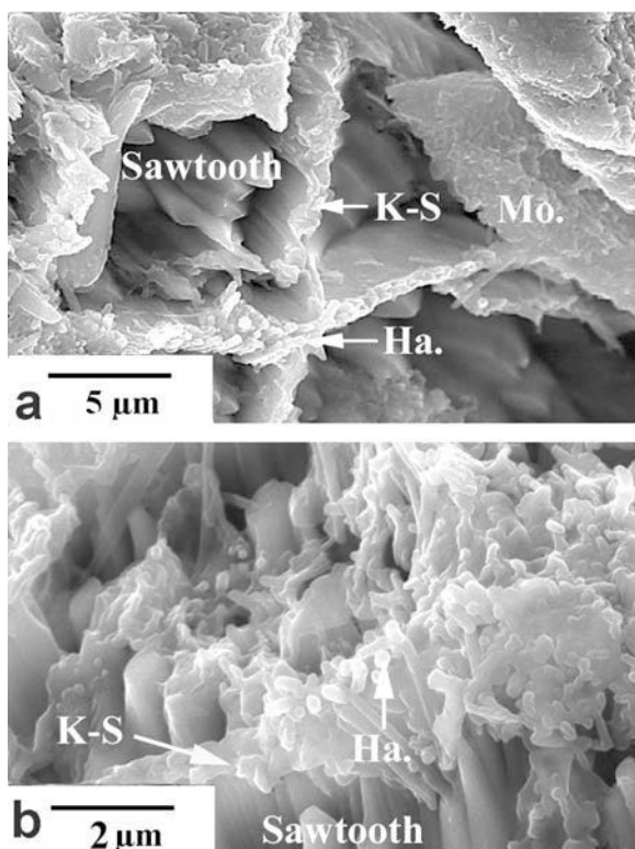
Figure 9. SEM images of a smectite, interstratified K-S and halloysite crystallization sequence on (001) planes of amphibole grains from sample 1: (a) mixed-layer K-S (K-S) and halloysite (Ha.) crystallization at the top of a sawtooth, covered with a montmorillonite (Mo.) honeycomb layer; (b) crystallization of halloysite (Ha.) on mixed-layer K-S (K-S).
