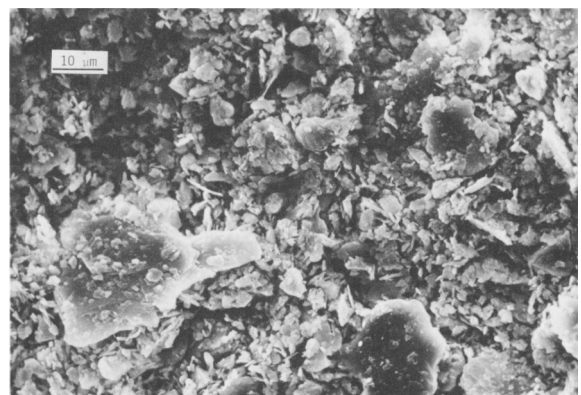
Figure 3. Scanning electron micrograph of suspended sediment from section G7. This representative micrograph illustrates the relation between particle size and mineralogy, the dominant fabric of the kaolinite, and the poorly sorted nature of the suspended sediment.
