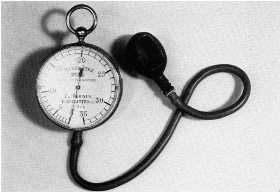
Figure 4 A Potain sphygmomanometer. Made by Charles Verdin of Paris. 5.1 cm diameter and graduated from 0–320 mm Hg, it lacks the side attachment for replenishing the air. It formerly belonged to Thomas Lauder Brunton. A600273.
