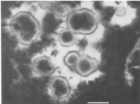
Figure 2. Backscattered-electron micrograph of cacoxenite aggregates showing distinct cores and overgrowths. Relative backscattered intensities indicate that cores have lower average atomic weight than overgrowths. Darkened areas in central portion of cores are topographic artifacts caused by the plucking of material during polishing of the sample surface. Bar is 10 \mu\text{m} .
