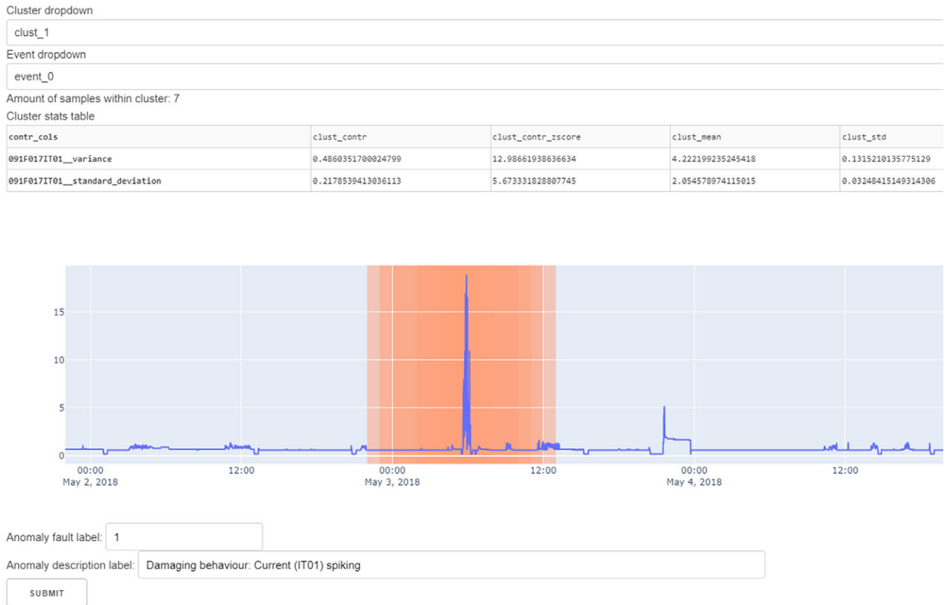
Figure 5. Example of the labeling dashboard with an anomaly of filter F017. This cluster of anomalies is caused by a current sensor having odd variance and standard deviation values within the window(s) shown in orange. Hence, the cluster is labeled by an expert as damaging behavior along with a small description.
