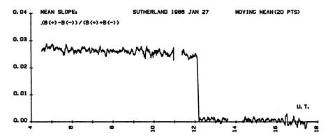
The variation of the slope of the 769.9 nm Fraunhofer absorption line of sunlight as it moves relative to the laboratory standard during the day is shown in the figure. The mean slope agrees within a few
