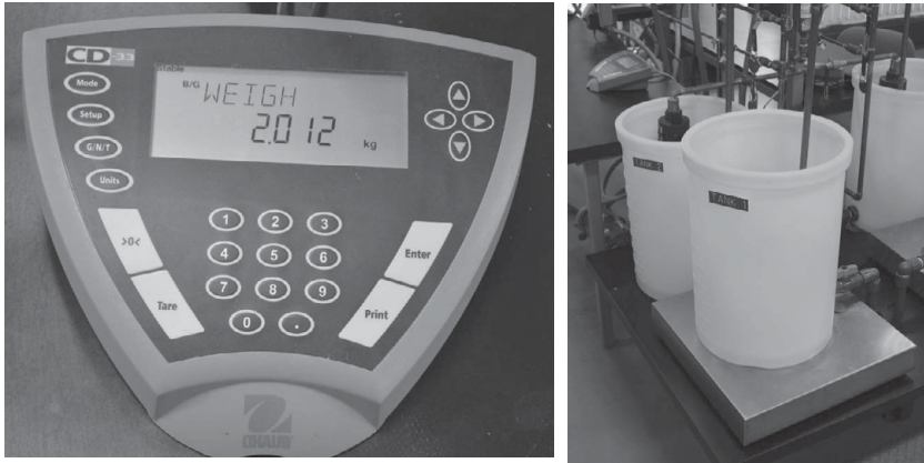
Figure 1.2 An electronic display (left) gives the reading from the scale underneath the water tank on the right. Displays from which we read data limit the precision of the measurement. This limitation contributes to reading error.
