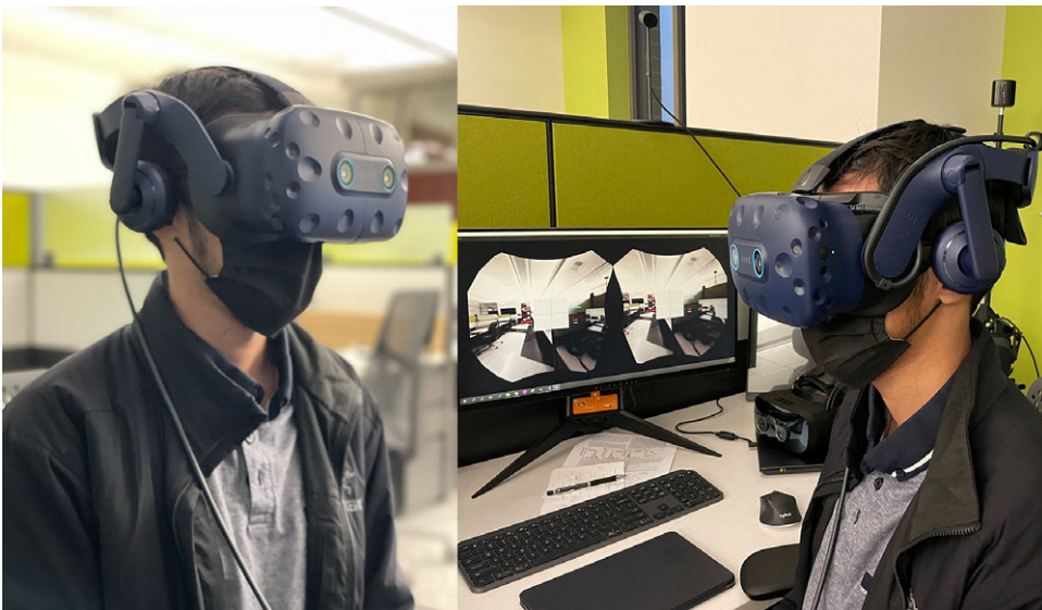
Figure 3. Hardware for the digital metamorphopsia suppression countermeasure. HTC Vive Pro Eye headset with user undergoing augmented reality with overlaying Amsler Grid.
