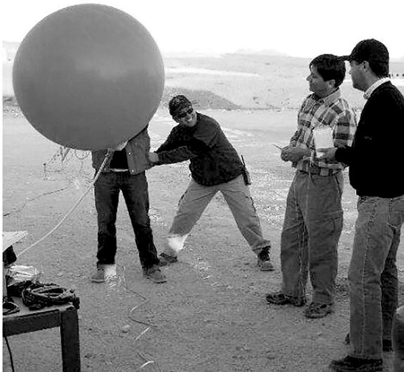
Figure 4.11 Launching a radiosonde balloon during an August 2005 study of the variation of atmospheric temperature across the ALMA site. Left to right: Rubén Bravo (behind balloon), Roberto Rivera, Angel Otárola, Jorge Riquelme. Courtesy of Alison Stirling, reproduced by permission.
