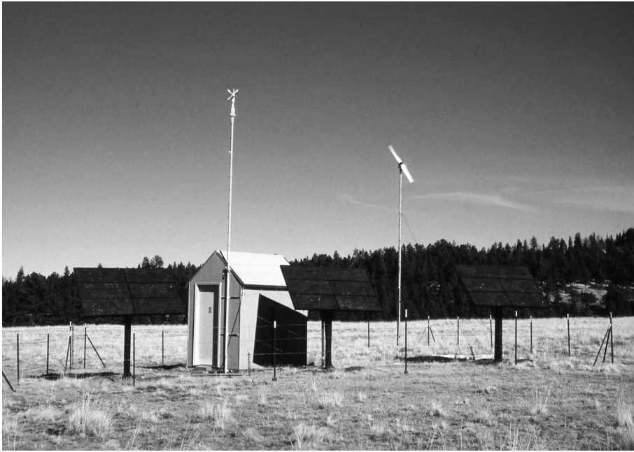
Figure 4.4 The weather station on the Springerville site. The shed held the tipping radiometer and recording equipment. Battery power was maintained by solar panels and a windmill. Credit: Frazer Owen, NRAO/AUI/NSF, CC BY 3.0.
