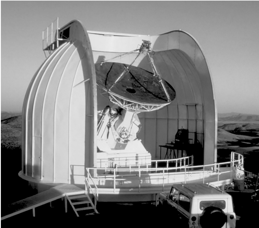
Figure B.1 The MWO 4.9 Meter Telescope in its renovated astro-dome equipped with an error-correcting subreflector. Credit: McDonald Observatory, University of Texas at Austin, reproduced by permission.
