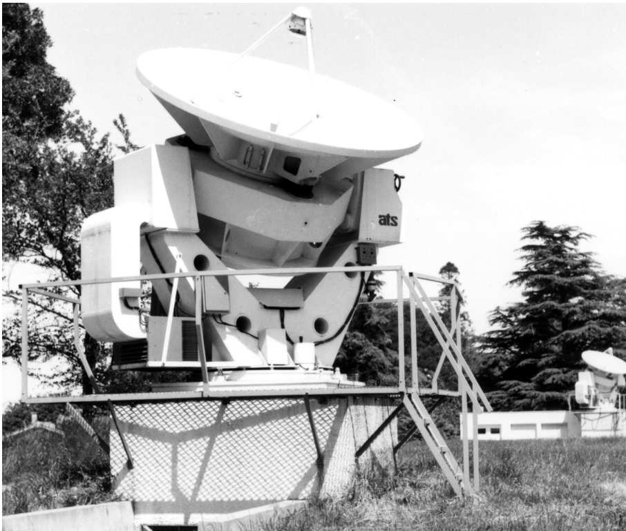
Figure 3.1 Photograph of the two-element interferometer built at the Observatoire de Bordeaux to observe the Sun. Courtesy of Alain Baudry, © Collection Observatoire Aquitain des Sciences de l'Univers, Laboratoire d'Astrophysique de Bordeaux, reproduced by permission.
