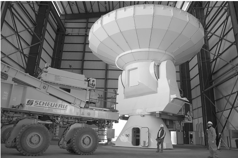
Figure 9.9 An antenna, ready for its electronics, being loaded onto a transporter. It is shown in the antenna assembly building, built by Vertex for assembly of its antennas. Credit: Art Symmes; NRAO/AUI/NSF, CC BY 3.0.
