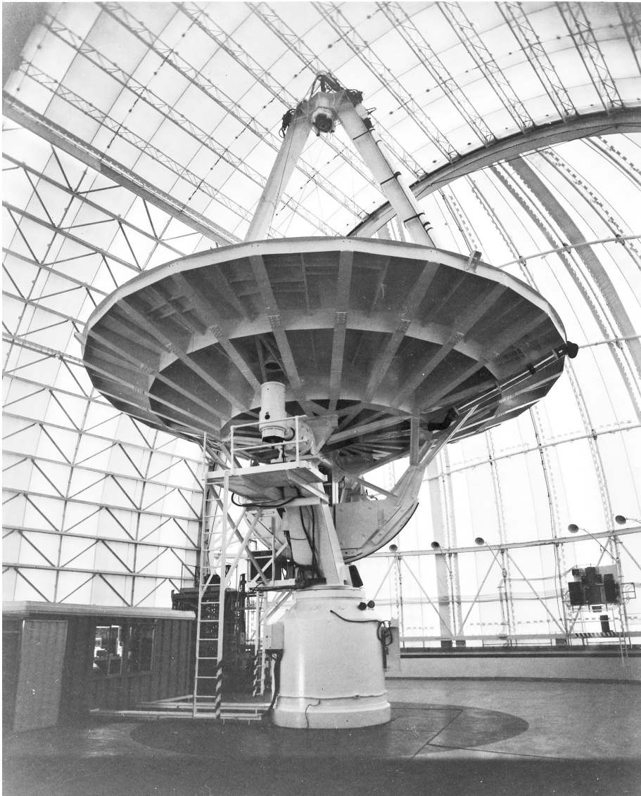
Figure 1.1 The NRAO 36 Foot Telescope in its fabric-covered astrodome on Kitt Peak, Arizona. Credit: NRAO/AUI/NSF, CC BY 3.0.
