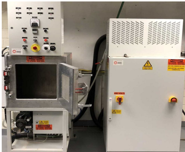
Fig. 1 Industrial microwave system (Thermex Thematron, 15 kW, 2.4 GHz).
