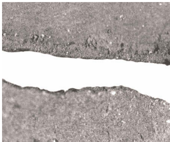
Figure 3. Optical micrographs (40 ×) of actual (above) and simulated (below) Type B solids.
