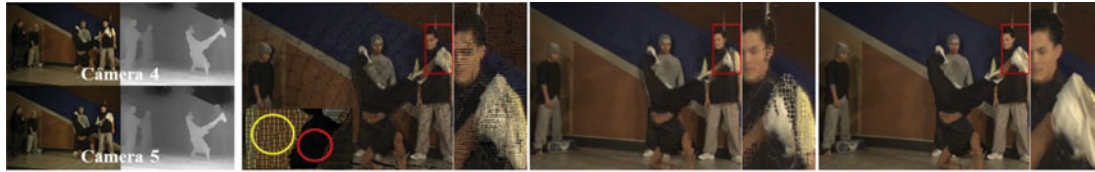
Fig. 1. Examples of synthesized virtual viewpoints. From left to right: input image + depth data (“breakdancers”, top: camera 4, bottom: camera 5), naive 3D warping [10], area highlighted with yellow circle shows the holes with limited sampling density, and area highlighted with red circle is disocclusion hole (right: close-up), MPEG view synthesis reference software, VSRS 4.0 [9] (right: close-up), and proposed method (right: close-up).
